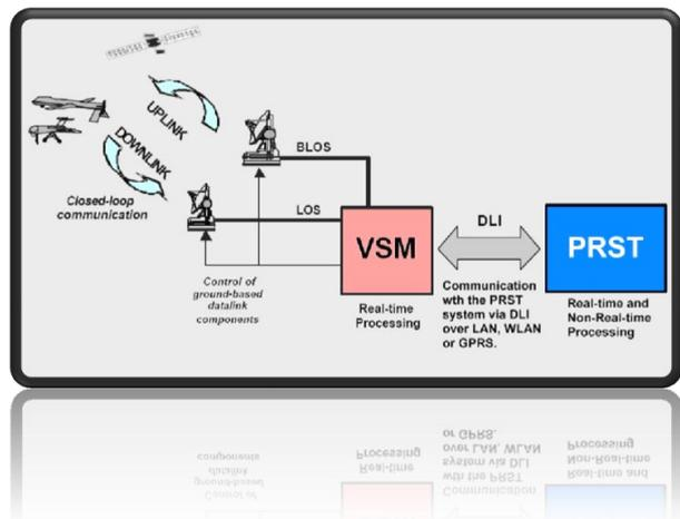
The custom VSM application communicates with the underlying data structures by interfacing directly with the API. The API in turn communicates with the CUCS. The API is using the UDP protocol for communication according to the STANAG 4586 specifications. As a result, you can develop an VSM application where all of the details regarding the underlying interactions have been abstracted away.
